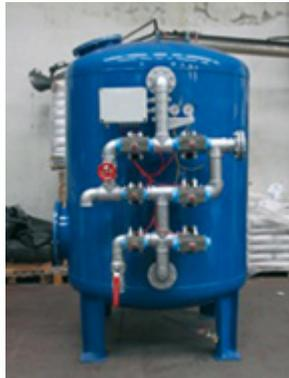
In its standard configuration, the filter is made of thick carbon steel sheeting and profiles with an outer epoxy coating and inner epoxy glaze suited to use with food; one or more inspection covers, supports, eyebolts for lifting, valves, nozzles, manometers and inlet and outlet pipes with fittings.
