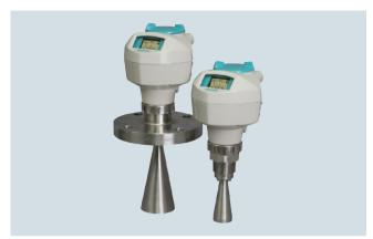
SITRANS LR250 is a 2-wire, 25 GHz pulse radar level transmitter for continuous monitoring of liquids and slurries in storage and process vessels including high temperature and pressure, to a range of 20 m (66 ft).
