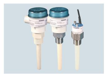
Pointek CLS100 is a compact 2-wire inverse frequency shift capacitance switch for level and material detection in constricted spaces, interfaces, solids, liquids, slurries and foam, with the ability to tune out build-up on probe.
