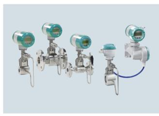
SITRANS F X vortex flowmeters provide accurate volumetric and mass flow measurement of steam, gases and liquids as an all-in-one solution with integrated temperature and pressure compensation.
