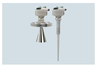
SITRANS LR200 is a 2-wire, 6 GHz pulse radar level transmitter for continuous monitoring of liquids and slurries in process vessels including high temperature, pressure, agitation, and turbulence to a range of 20 m (65 ft).
