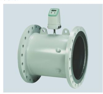
The 2-path flowmeter SITRANS FUE380 comes as battery or mains-powered and is designed to measure water flow in district heating plants, local networks, boiler stations, substations, chiller plants and other general water applications.
