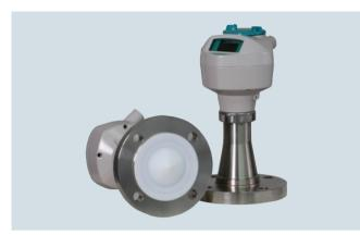
SITRANS LR250 with flanged encapsulated antenna is a 2-wire. 25 GHz pulse radar level transmitter for continuous monitoring of liquids and slurries in storage and process vessels including corrosives or aggressive materials, to a range of 20 m (66 ft) (antenna dependent).
