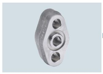
The oval flange 7MF9408-2C. for pressure transmitters for absolute pressure and differential pressure has a  $\frac{1}{2}$ -14 NPT female thread and is designed for max. operating pressure 400 bar (5800 psi).
