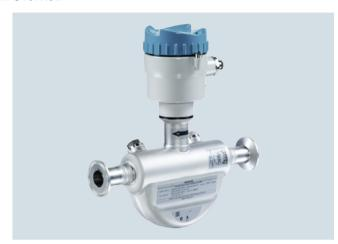
The flow measuring principle is based on the Coriolis Effect. The FCS400 sensor's measuring tubes are energized by an electromechanical driver circuit which oscillates them at their resonance frequency.
