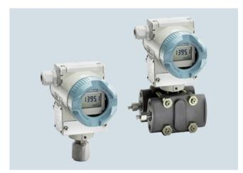
SITRANS P410 pressure transmitters are digital pressure transmitters with a high level of operating convenience. Technically, they are based on the SITRANS P DS III but offer an increased measuring accuracy of 0.04%. This means the SITRANS P 410 is perfectly suited for measuring tasks with increased accuracy requirements. The parameterization is performed using input buttons or via HART or via PROFIBUS PA or FOUNDATION Fieldbus interface.
