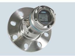
SITRANS LR560 2-wire, 78 GHz FMCW radar level transmitter for continuous monitoring of solids in silos to a range of 100 m (329 ft).
