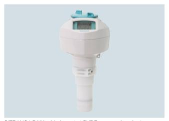
SITRANS LR250 with threaded PVDF antenna is a 2-wire, 25 GHz pulse radar level transmitter for continuous monitoring of liquids and slurries in storage and process vessels including corrosives or aggressive materials, to a range of 10 m (32.8 ft) or 20 m (66 ft) when used in a stilling pipe.
