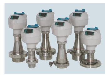
The SITRANS LR250 hygienic encapsulated antenna is a 2 wire 25GHz pulse radar level transmitter with sanitary and hygienic approvals for continuous monitoring of liquids, slurries and pastes within the Food, Beverage, chemical, and pharmaceutical industries to a range of 20 m (66 ft) - antenna dependent. (Pictures shown with accessories - sold separately)
