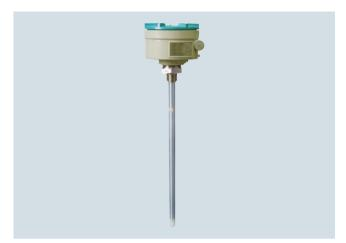
Pointek CLS500 is an inverse frequency shift capacitance level and material detection switch ideal for detecting interfaces, solids, liquids, toxic, and aggressive chemicals in critical conditions of high temperature and pressure. CLS500 also has the ability to tune out build-up on the probe.
