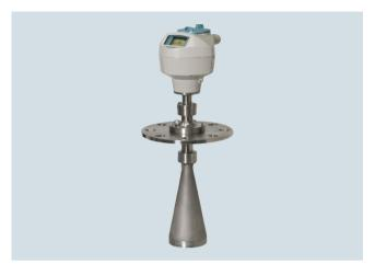
SITRANS LR260 is a 2-wire 25 GHz pulse radar level transmitter for continuous monitoring of solids and liquids in storage vessels including extreme levels of dust and high temperatures, to a range of 30 m (98.4 ft).
