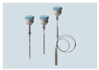
Pointek CLS300 (standard version) is an inverse frequency shift capacitance level and material detection switch with optional rod/cable choices and configurable output. CLS300 is ideal for detecting liquids, solids, slurries, foam, and interfaces in demanding conditions where high pressure and temperatures are present and has the ability to tune out build-up on the probe.
