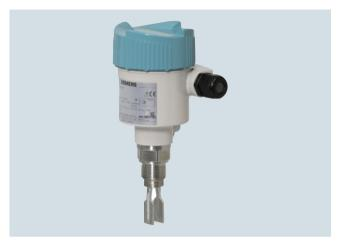
SITRANS LVL200 is a standard vibrating level switch for material detection in liquid and slurry applications such as overflow, high, low, and demand applications, as well as pump protection. For use in SIL 2 applications.
