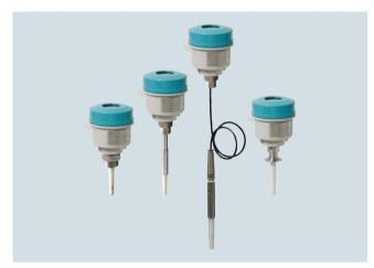
Pointek CLS200 (digital version) is a versatile inverse frequency shift capacitance level and material detection switch with optional rod/cable choices and configurable output. CLS200 is ideal for detection of liquids, solids, slurries, foam and interfaces and has the ability to tune out build-up on the probe. The digital version includes PROFIBUS PA, an LCD display, and advanced diagnostic features.
