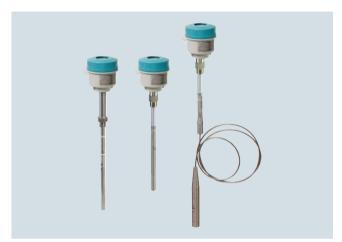
Pointek CLS300 (digital version) is an inverse frequency shift capacitance level and material detection switch with optional rod/cable choices and configurable output. It is ideal for detecting liquids, solids, slurries, foam and interfaces in demanding conditions where high pressure and temperatures are present and has the ability to tune out build-up on the probe. The digital version includes PROFIBUS PA, an LCD display, and advanced diagnostic features.
