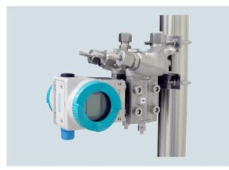
The 3-way valve manifold DN 8 (7MF9416-1../-2..) is for pressure transmitters for differential pressure. It is used to shut off and blow out differential pressure lines and to test the pressure transmitter zero.
