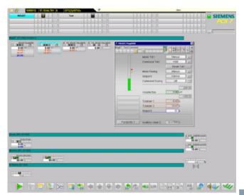
The SITRANS Library for SIMATIC PCS 7 V8.0 and higher extends standard functionality of the SIMATIC PCS 7 process control system concentrated in the SIMATIC PCS 7 Advanced Process Library (APL) with technological blocks and faceplates for device-specific functions of the SITRANS field devices.
