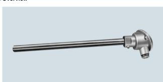
The straight thermocouple together with a metal protective tube is suitable for temperatures from 0 to 1250 °C (32 to 2282 °F) and can be supplied with a built-in temperature transmitter.
