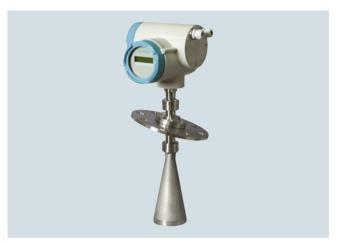
The SITRANS LR460 is a 4-wire, 24 GHz FMCW radar level transmitter with extremely high signal-to-noise ratio and advanced signal processing for continuous monitoring of solids up to 100 m (328 ft). It is ideal for measurement in extreme dust.
