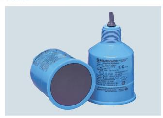
EchoMax XRS-5 ultrasonic transducer provides reliable, continuous level monitoring of liquids and slurries in narrow lift stations/wet wells, flumes, weirs and filter beds using a beam angle of just 10° and a CSM rubber face.
