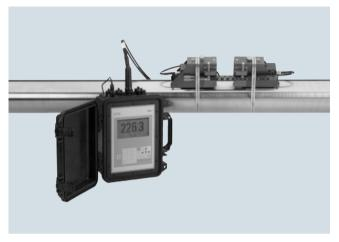
SITRANS FUP1010 clamp-on non-intrusive ultrasonic flow transmitter offers maximum versatility plus battery power for portable field use. It can operate in either WideBeam transit time or reflexor (Doppler) mode, making it suitable for virtually any liquid, even those with high aeration or suspended solids.
