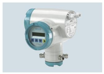
SITRANS FUS060 is a transit time based transmitter designed for ultrasonic flowmetering with dedicated sensors in the FUS inline series up to DN 4000. SITRANS FUS060 is engineered for high performance and is suitable for 1-path, 2-path and 4-path flowmeters.
