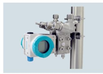
The three-spindle and five-spindle valve manifolds DN 5 (7MF9410-1../-3..) are used to shut off the differential pressure lines and to check the transmitter zero.
